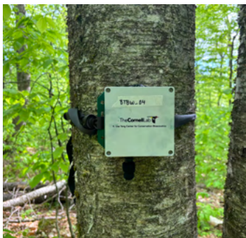
Autonomous recording unit (ARU) from the Cornell Lab of Ornithology, passively recording acoustic data.
